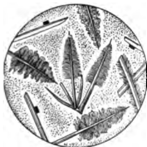
FIG. 223. Microsection showing the Beginnings of Crystal Growth in Glassy Lava
